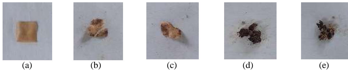
Figure 15 The physical appearances of SCB 3 bioplastic; (a) before burial test, (b) after two days, (c) after four days, (d) after six days and (e) after eight days burial
